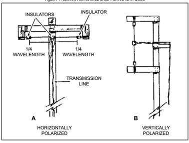
(b) The half-wave antenna is used with FM radios (Figure 7-8). It is effective in heavily wooded areas to increase the range of portable radios. Connect the top quidelines to a limb or pass it over the limb and connect it to the tree trunk or a stake.
