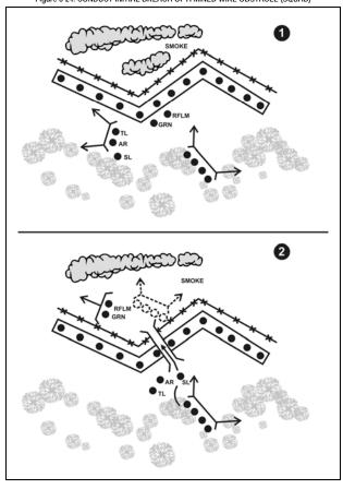
Figure 6-25. CONDUCT INITIAL BREACH OF A MINED WIRE OBSTACLE (PLATOON) MORTAR SMOKE SMOKE
