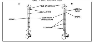
Figure 7-1. USE OF BROKEN ANTENNA
