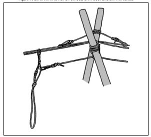
Figure 10-27. SUSPENSION TRAVERSE
