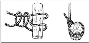
c. End-of-the-Rope Clove Hitch. The end-of-the-rope clove hitch (Figure 10-7) is an intermediate anchor knot that requires constant tension. Make two turns around the anchor. A locking bar runs diagonally from one side to the other. Leave no more than one rope width between turns of rope. Locking bar is opposite direction of pull. When you dress the knot, leave at least a 4-inch tail on the working end.
