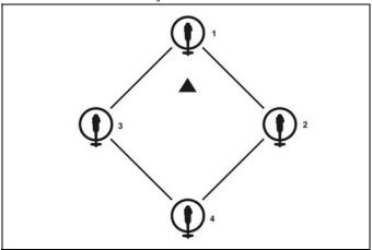
c. Vee. Requires a relatively small landing area; allows rapid deployment of forces to the front; restricts suppressive fire of inboard gunners; presents some difficulty in pre-positioning loads (Figure 8-4).
