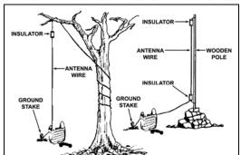
Figure 7-3. VERTICAL ANTENNA MADE FROM A WIRE SUPPORTED BY A TREE OR WOODEN POLE
