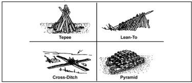
(2) Cross-Ditch (Figure 11-19). Scratch a cross about 1 foot in size in the ground. Dig the cross 3 inches deep. Put a large wad of tinder in the middle of the cross. Build a kindling pyramid above the tinder. The shallow ditch allows air to sweep under the fire to provide a draft.
