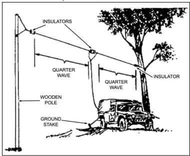
Figure 7-6. CENTER-FED, DOUBLET ANTENNA
