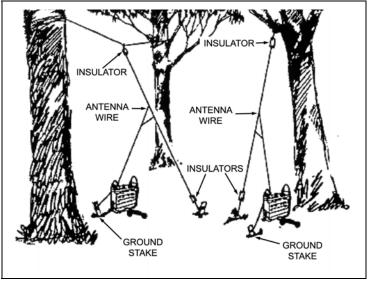
Figure 7-8. HALF-WAVE ANTENNA USED WITH FM RADIO
