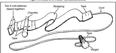
Figure 14-2. EXAMPLE OF A WOLF-TAIL MARKING DEVICE
