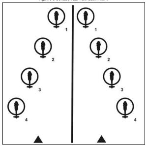
e. **Trail**. Requires a relatively small landing area; allows rapid deployment of forces to the flank; simplifies pre-positioning loads; allows unrestricted suppressive fire by gunners (Figure 8-6).
