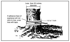
Figure 13-12. TIMBER-CUTTING CHARGE (EXTERNAL)
